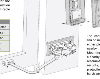
The control panel can be mounted on either pier, or on a nearby wall. Mounting it inside a nearby garage, is recommended for security, and protection from harsh weather.
