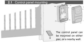
Wiring and programming is covered in another document. Mains cables should be protected in ducts or armmoured sheathing. All other cables are ELV designated electrically safe.
